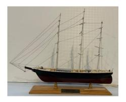
Clipper ships were designed to compete for the passenger and cargo trade going from the east to the west coast, around Cape Horn. They had new and original naval design characteristics that were meant for speed: long and narrow hulls, narrow cutting bows, low freeboard, streamlined sterns, and large amounts of sail.
