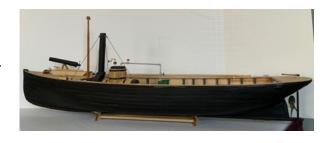
Spar Torpedo Boats were invented during the U.S. Civil War. They were small steamboats (approximately 45' long and 9' feet wide) fitted with a 'spar torpedo', which is a bomb (torpedo) that was attached to the end of a long pole (spar). The steamboat would take aim at an enemy ship and when it was close enough, it would ram the vessel and drive the long spar into it, and then detonate the torpedo at the end of the spar.
